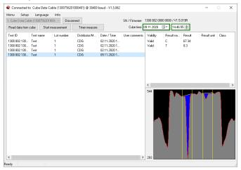
All information concerning the demo measurement can be seen, OEM information, measurement result values and the 2D volume diagram.
