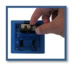
After three AA batteries have been placed in the holder it needs to be reinserted into the reader. The holder only fits one way with the round corners pointing towards the back of the device. An anti-twist safeguard will protect a wrong insertion sidewise. If the holder seems to clamp within the slot please turn the adapter and try the insertion again. A "click" sound will appear when the adapter has been inserted completely and correctly.
