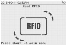
If the RFID tag is attached to the cartridge this screen will only show up for less than 1s and the measurement information screen will be displayed. If not, the reader will wait for four minutes before showing an error
