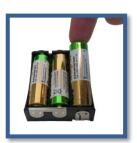
If no batteries are inserted in the holder or if the batteries need to be changed new batteries need to be placed in the holder. Follow the marks on the holder to ensure correct polarity ('+'- sign up, see Fig.). Add the batteries one by one.
