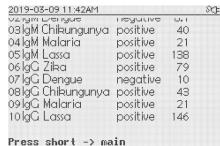
The result includes a result number, the result name, the class (if setup in the configuration file) and the measured value.
